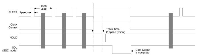
Figure 2. Timing for "shallow sleep" function (Timing segments not to scale).
